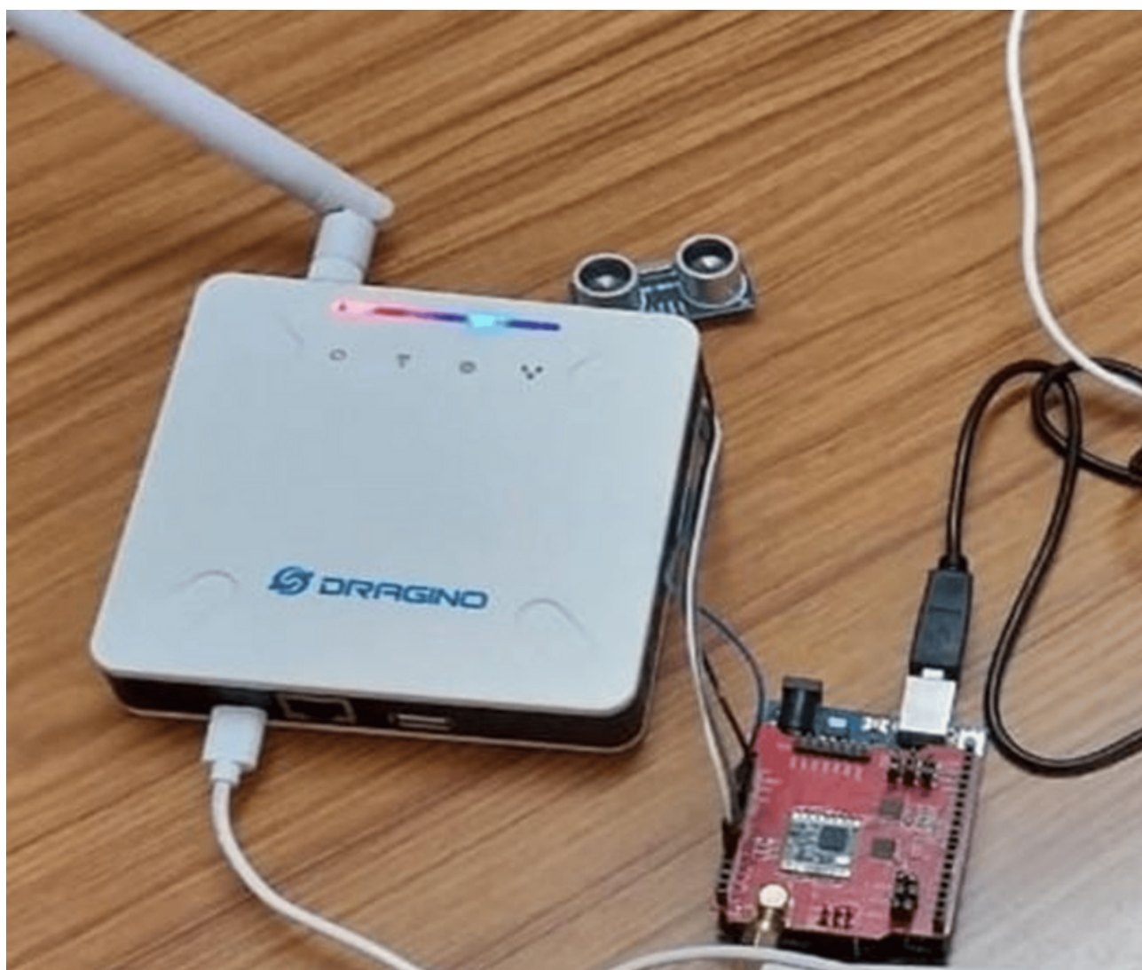
FIGURE 5: Hardware test of canal obstruction detection using LoRa
