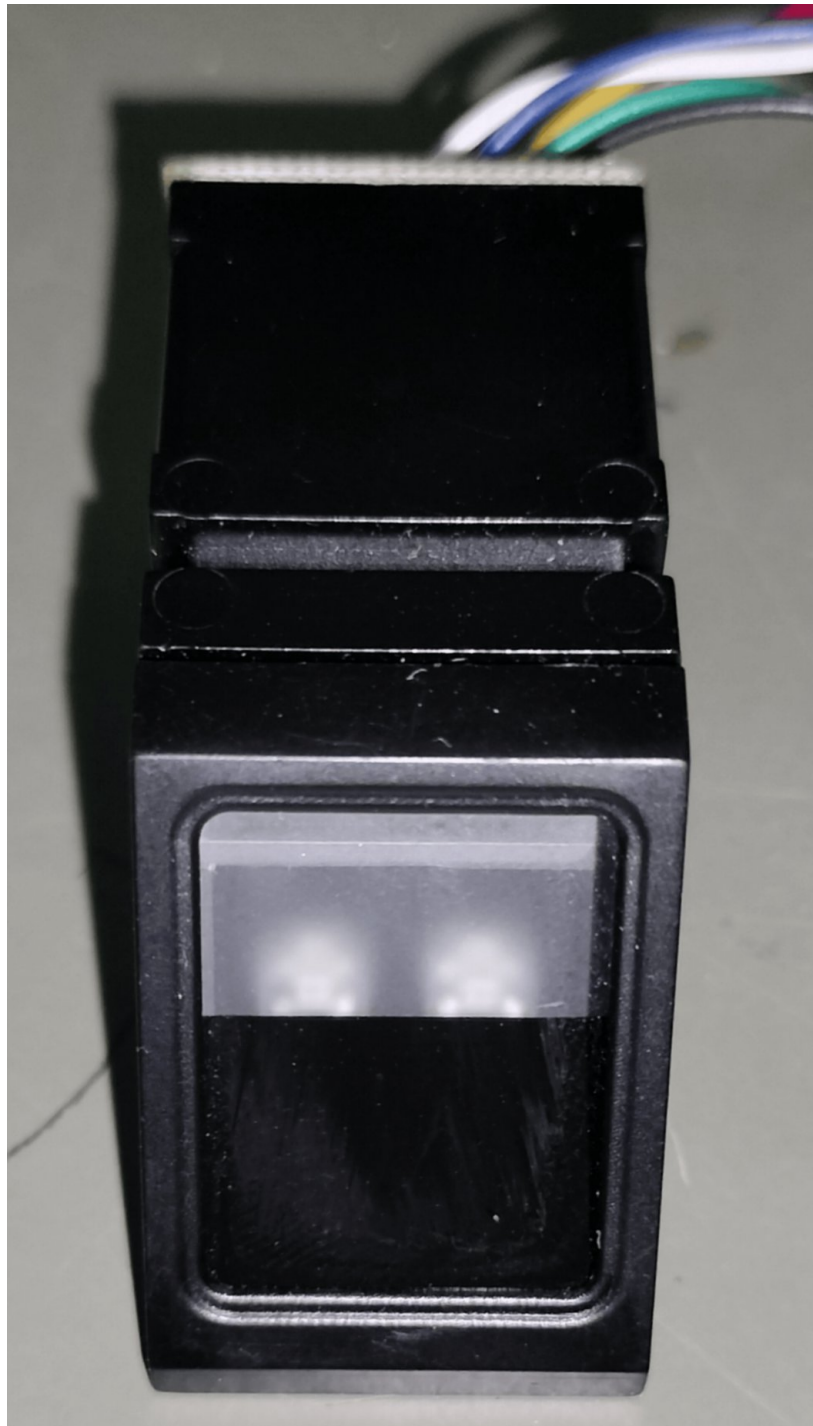
FIGURE 3: R307 fingerprint sensor module
