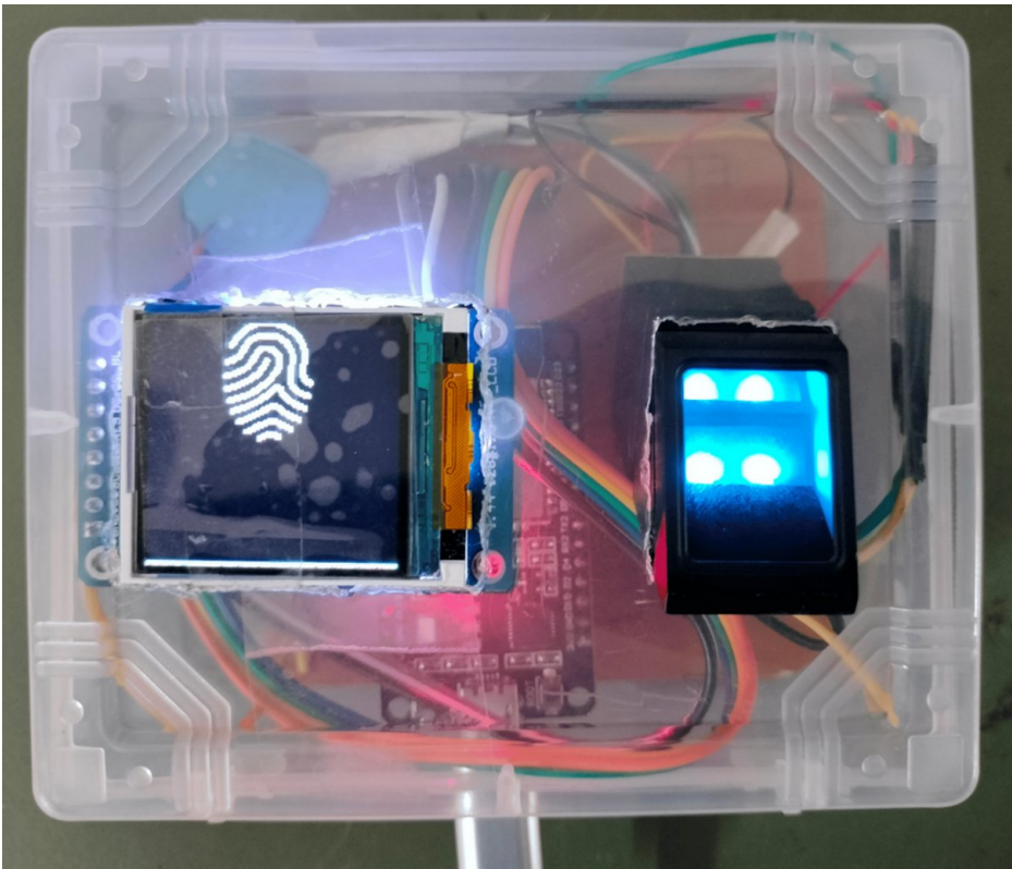
FIGURE 11: Front view of the developed portable smart attendance system
