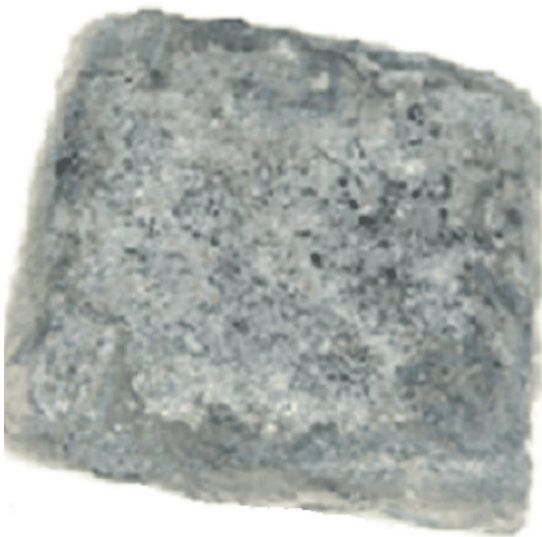
FIGURE 33: TA pieces laid aluminium plate with TIPC coatings after heat flux tests TA, tungsten alloy; TIPC, thermal insulation polyimide composite
