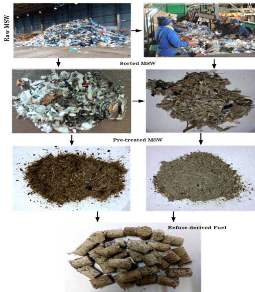
FIGURE 1: Production of refuse-derived fuel (RDF) from raw MSW
