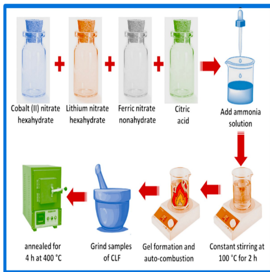
FIGURE 1: Experimental detail of synthesis of \text{LiCo}_x\text{Fe}_{2-x}\text{O}_4 where x : 0.0, 0.025, 0.050, and 0.075
