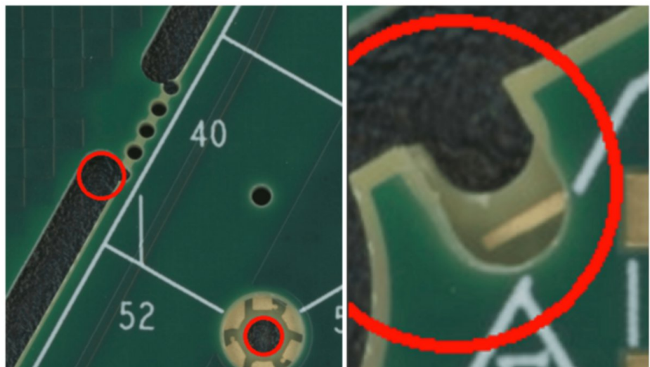
FIGURE 1: Examples of False Positive Detections Recorded During Initial Testing of Approach I. A Total of 13 False Positives Were Observed, Primarily Along PCB Edges or Irregular Contours, Representing Approximately 12.38% of Total Detections
