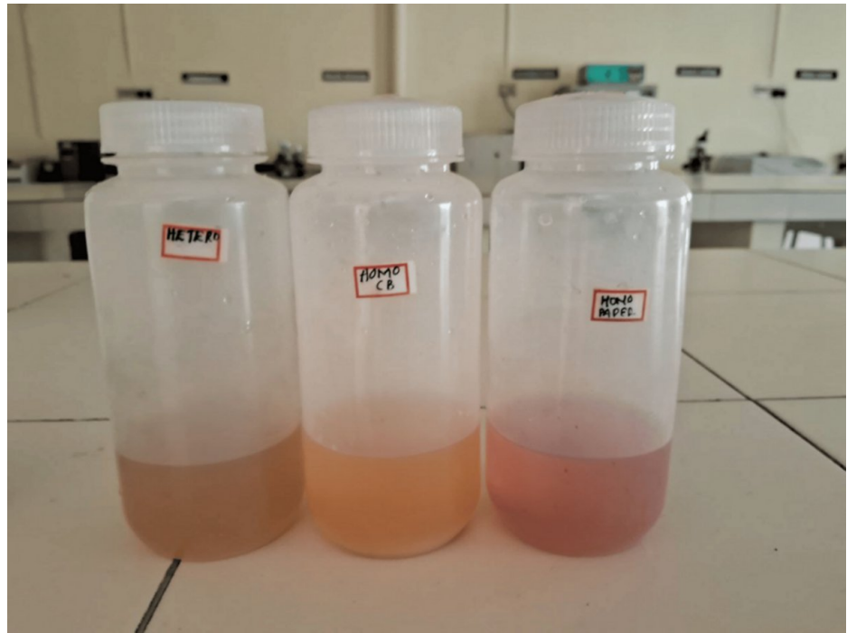
FIGURE 1: Substrate sample following acid pretreatment
