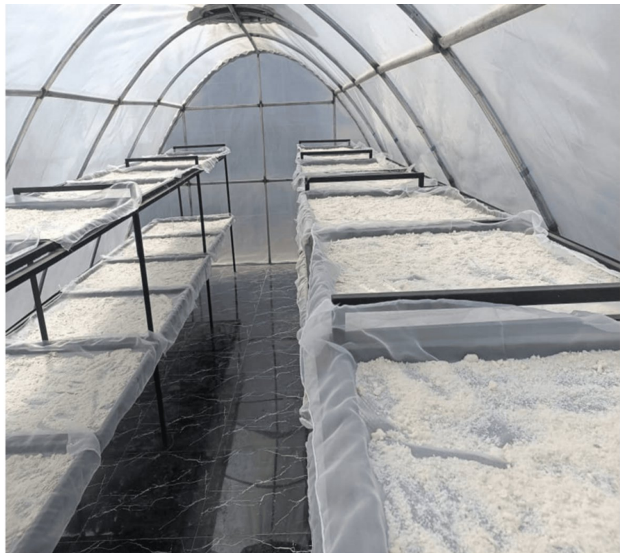
FIGURE 2: Drying of high-quality cassava flour using NSPRI PSSD
