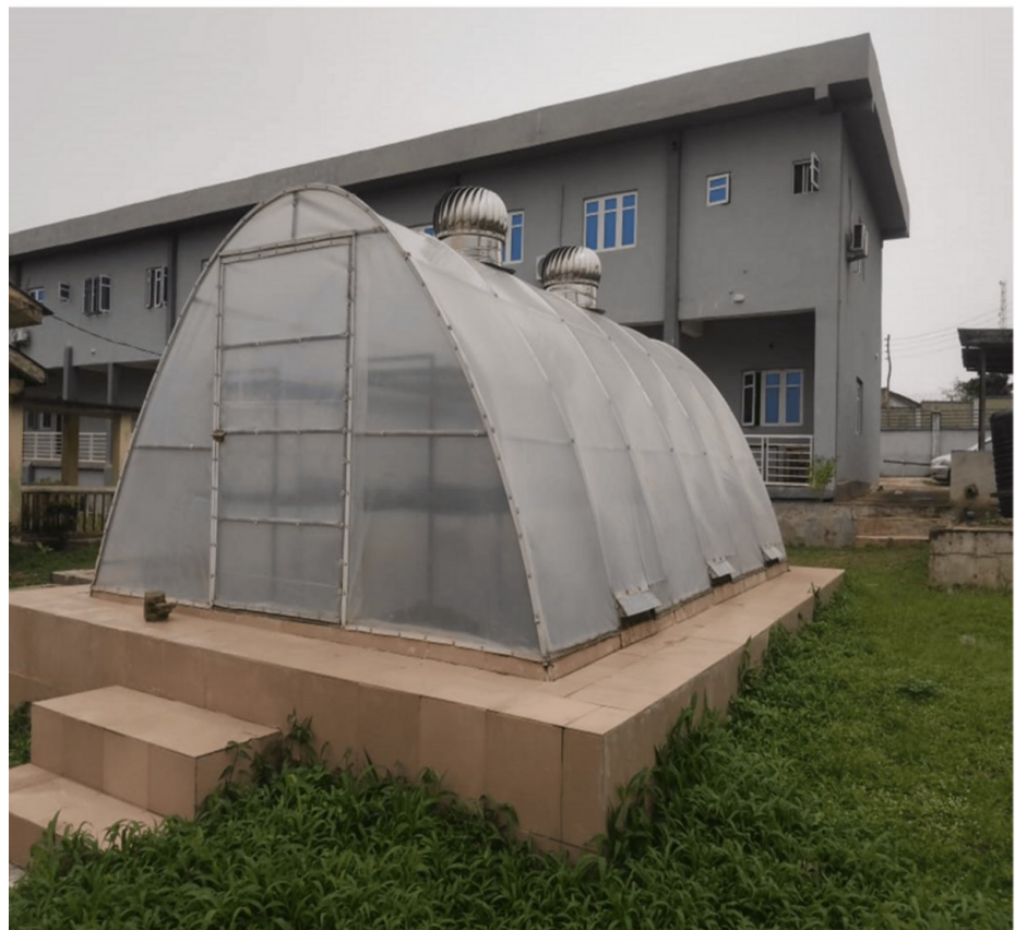
FIGURE 1: NSPRI parabolic-shaped solar dryer
