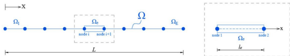
FIGURE 7: Finite element discretization of nanobeam and e-th finite element with corresponding degrees of freedom
