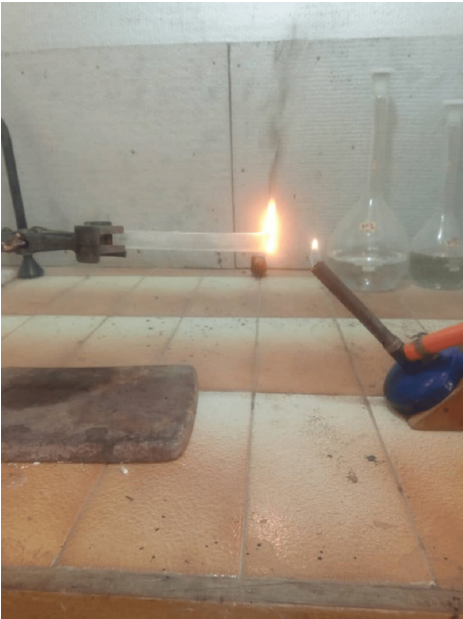
FIGURE 5: Flame propagation for control sample 0/0/100 wt.%
