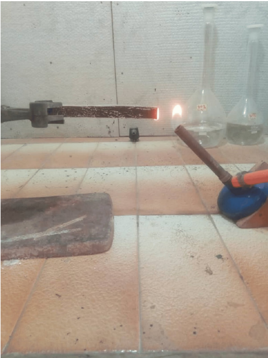
FIGURE 3: Flame propagation for hybrid sample 13/27/60 wt.%
