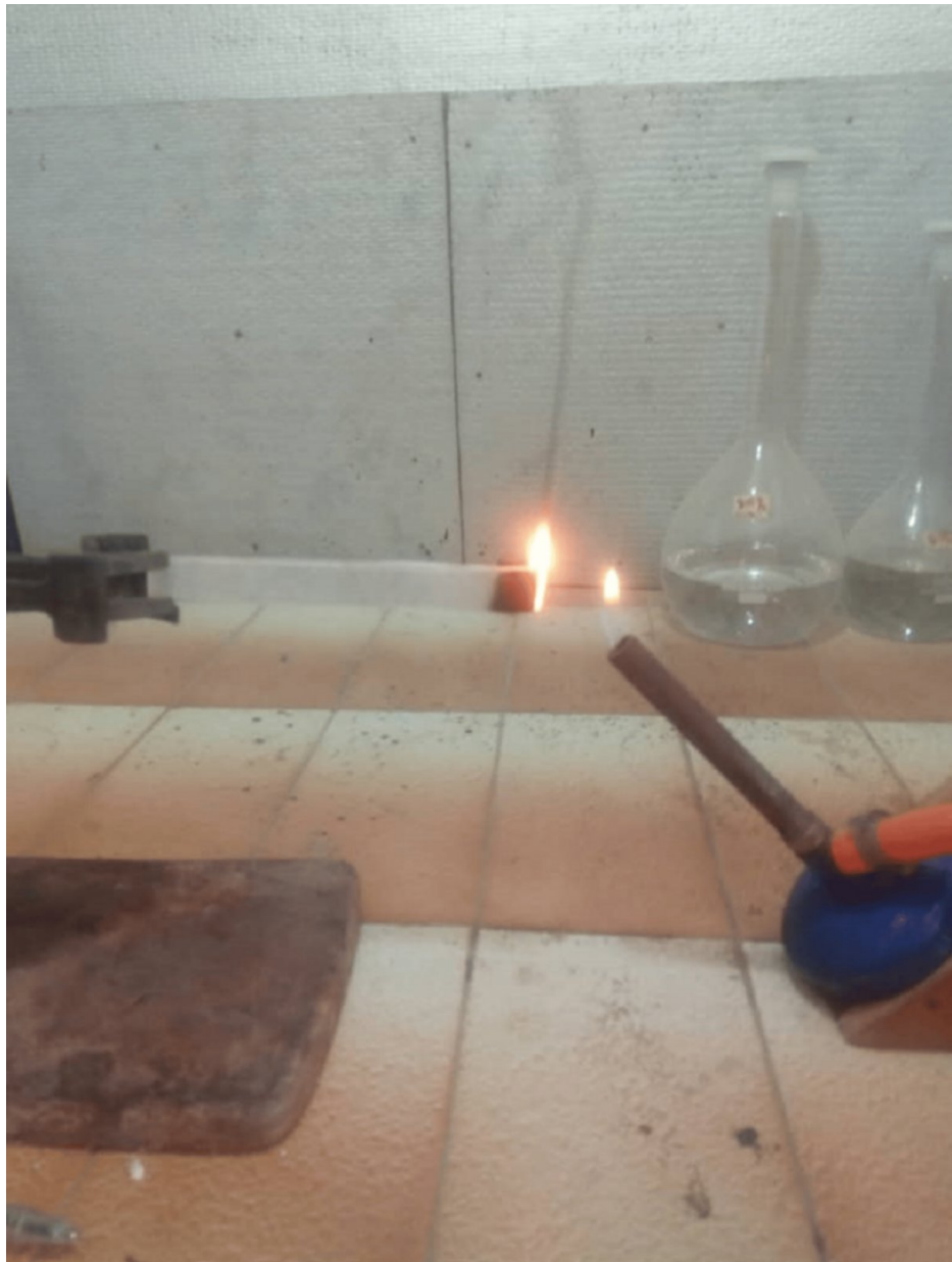
FIGURE 6: Flame propagation for glass reinforced sample 0/40/60 wt.%
