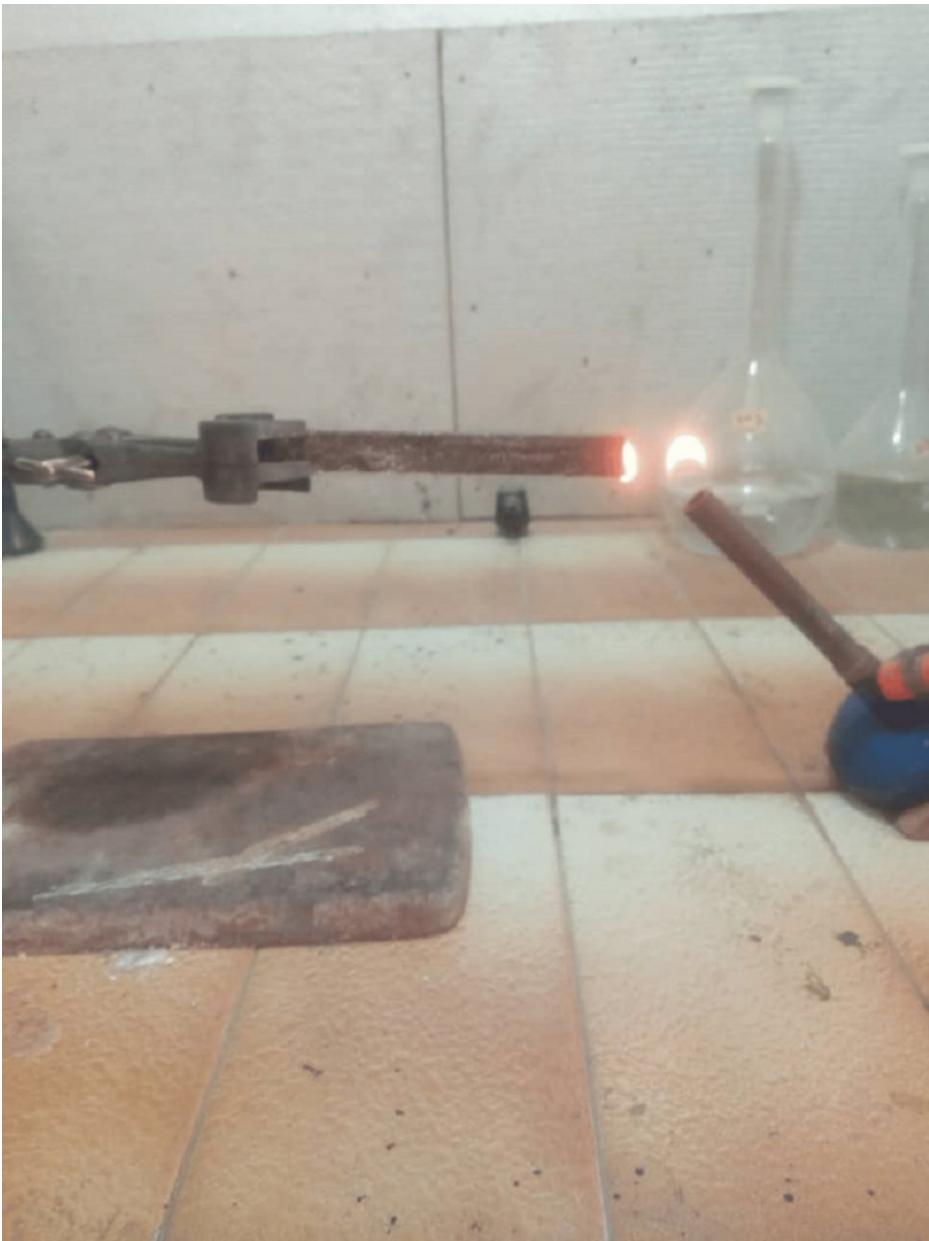
FIGURE 4: Flame propagation for hybrid sample 20/20/60 wt.%
