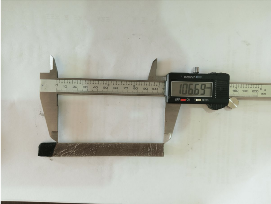
FIGURE 2: Measurement of extent of burning
