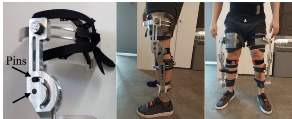
FIGURE 8: Left: The rotational pins of the knee exoskeleton, middle: KneExo worn by the healthy subject—side view, Right: KneExo worn by the healthy subject—front view
