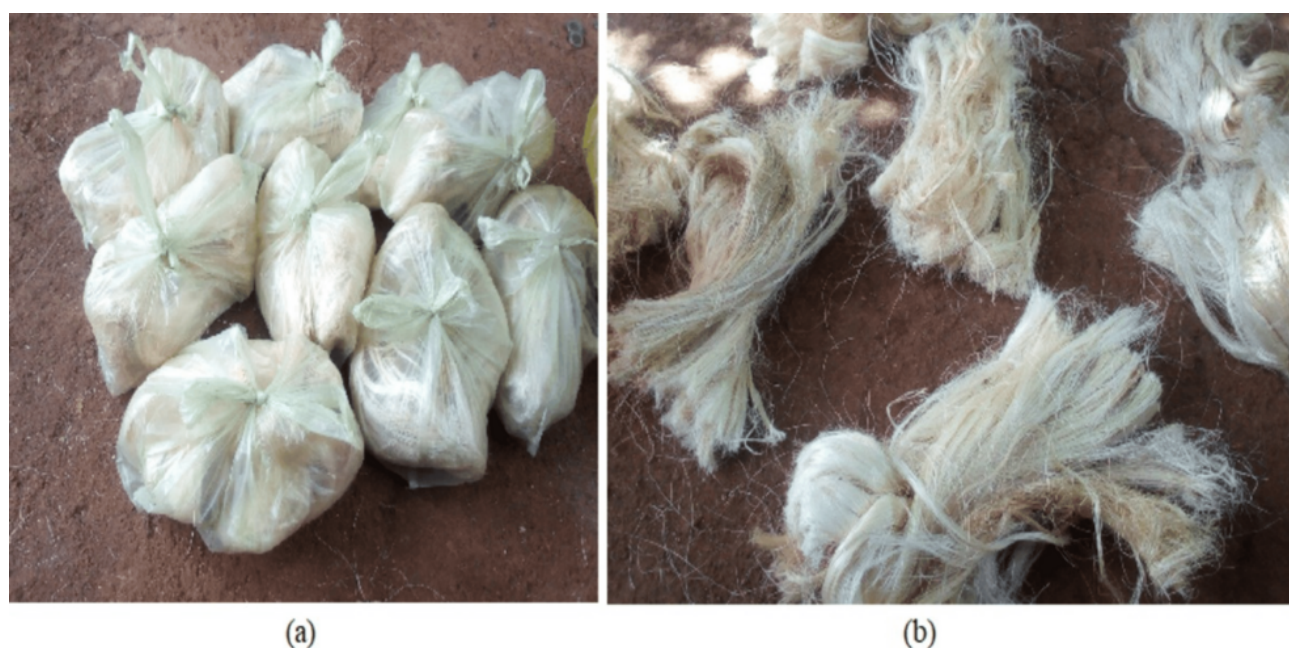
FIGURE 5: Sixty grams of packed jute fiber (a) and chopped jute fiber (b) before mixing
