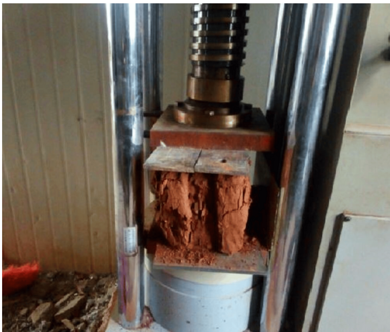
FIGURE 7: Adobe sample testing using a compression machine
