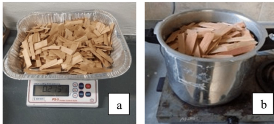
FIGURE 2: Preparation of wood strands from veneer leftovers
