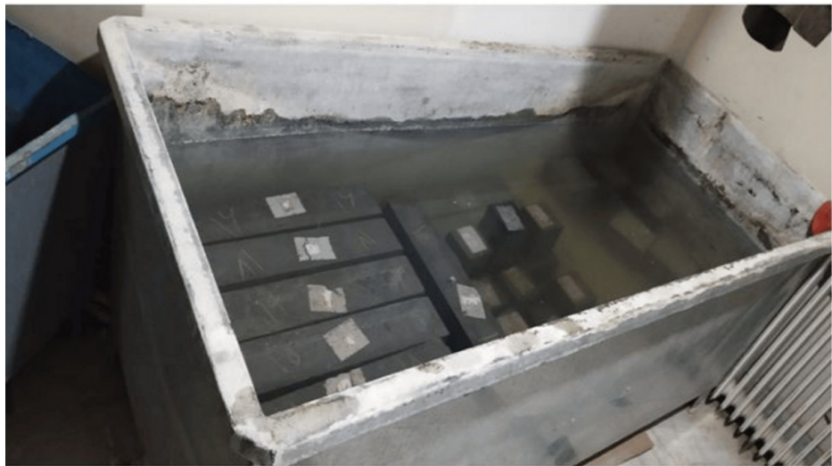
FIGURE 4: Curing of concrete samples in a curing water tank at a temperature of 18-22 degrees Celsius according to BS-1881 standard
