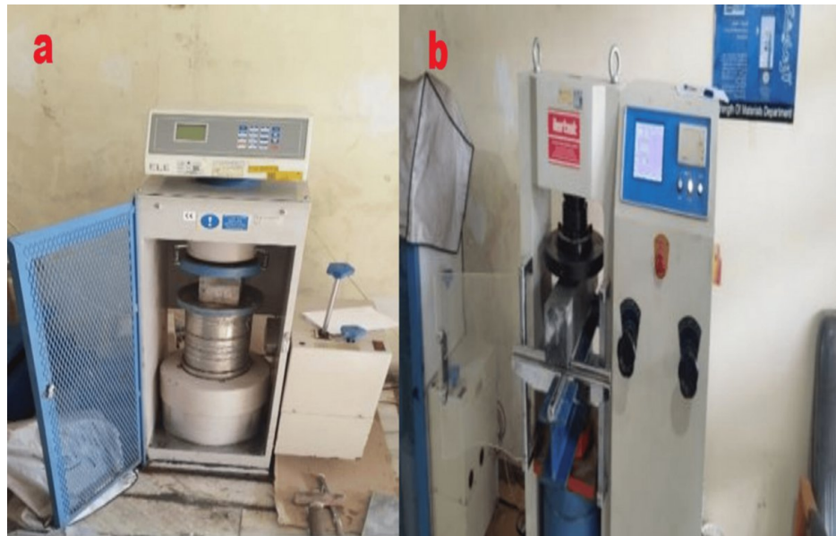
FIGURE 6: (a) Digital concrete breaker jack according to BS-1881 standard, (b) performing a flexural strength test according to ASTM C293 standard
