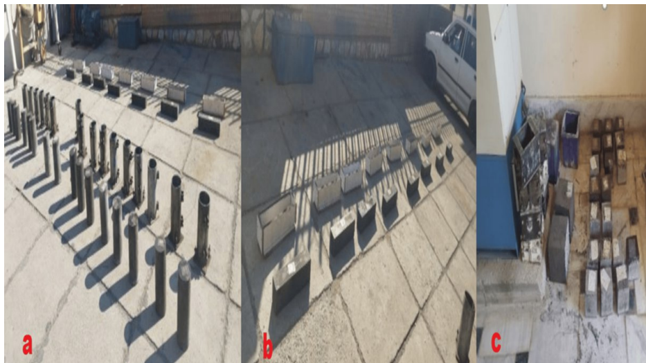
FIGURE 5: Image of (a) tensile, compressive, flexural, and impact strength test samples (before cutting), (b) flexural strength test specimens, (c) compressive strength test specimens
