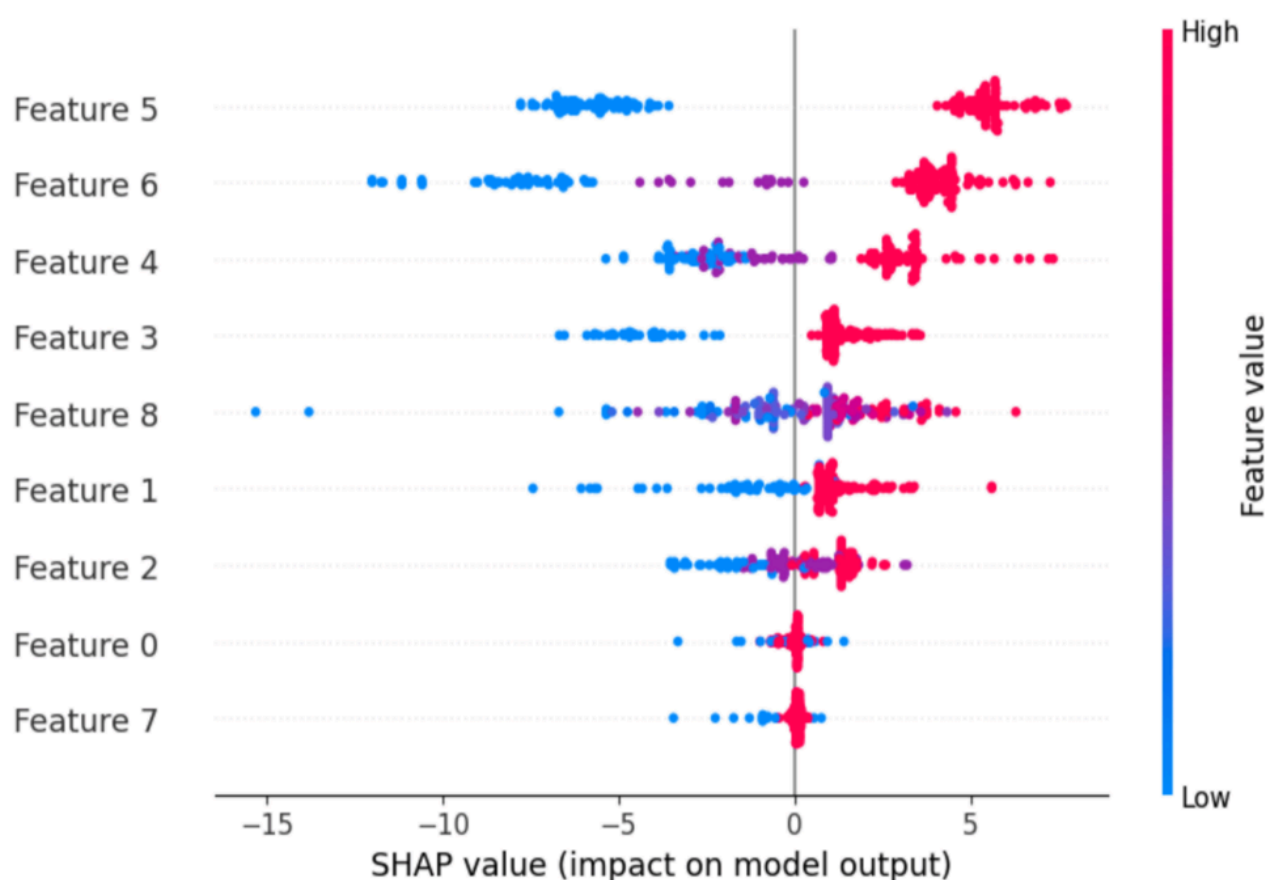
FIGURE 11: SHAP summary plot that displays the impact of each feature on the model's output. Each point represents a SHAP value for an instance, with colour representing feature value (blue for low and red for high). Features are ranked by importance, with higher absolute SHAP values indicating stronger influence.
