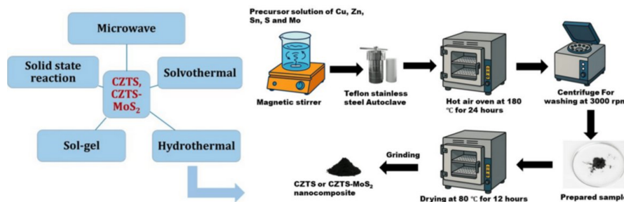
FIGURE 1: Schematic diagram of the synthesis process for CZTS and CZTS-MoS 2 nanocomposite
