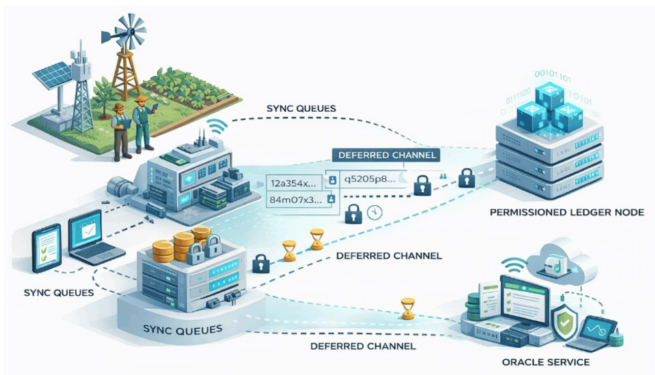
FIGURE 11: TRL 4–6 integrated architecture: addition of an edge gateway, synchronization queues, a permissioned ledger node, an oracle service, and an ESG/accounting validation module enabling auditable checks
